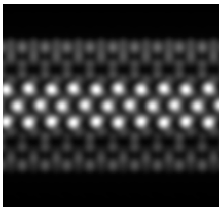
Figure 1. Simulated TEM image of SnTe nano-wire embedded in SWCNT
